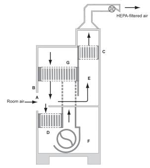
**Figure 5B.** *The Class II, Type B1 BSC (bench top design)* (A) front opening; (B) sash; (C) exhaust HEPA filter; (D) supply plenum; (E) supply HEPA filter; (F) blower; (G) negative pressure exhaust plenum. *Note:* The cabinet exhaust needs to be hard connected to the building exhaust system.
