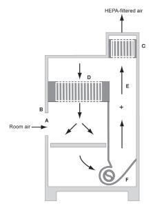
**Figure 4.** *Canopy (thimble) unit for ducting a Class II, Type A BSC* (A) balancing damper; (B) flexible connector to exhaust system; (C) cabinet exhaust HEPA filter housing; (D) canopy unit; (E) BSC. *Note:* There is a 1" gap between the canopy unit (D) and the exhaust filter housing (C), through which room air is exhausted.
