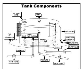
pumps fail to shut off. A screen or a closefitting flapper gate is required on the overflow to keep out birds, bugs, and mammals.
