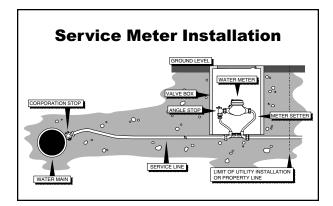
These meters are used to determine the amount of water sold. They also are used to determine unaccounted-for water and to identify leaks.
