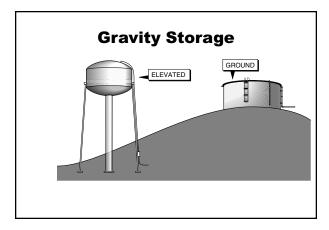
Large-Diameter Tanks Preferred. When gravity storage is used, the pressure at the head of the distribution system fluctuates with the water level in the tank. Shallow, large-diameter storage tanks are preferred over deep, small-diameter tanks because the larger diameter tanks have more water per foot of drawdown and are thus less prone to pressure fluctuations.
