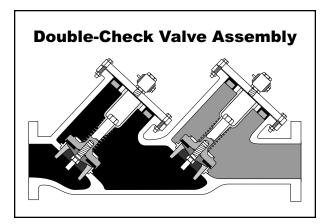
The double-check system has the advantage of a low head loss (maximum 10 psi). With the shut-off valves wide open, the two checks, when in an open position, offer little resistance to flow.
