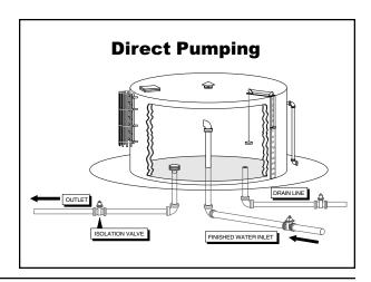
Water may also be pumped into the distribution system several miles from the tank, with the tank riding or **floating** on the system.
