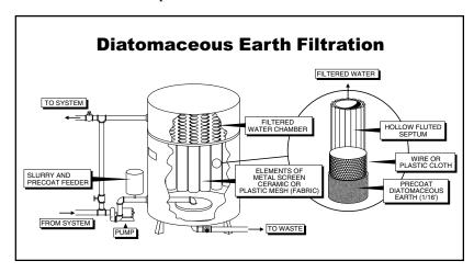
odor can be expected. The inspector should determine whether this facility has taste and odor problems that are attributable to long filter runs or prechlorination? How often is the septum inspected and cleaned (~100 filter runs)? How is the spent filter cake disposed of?
