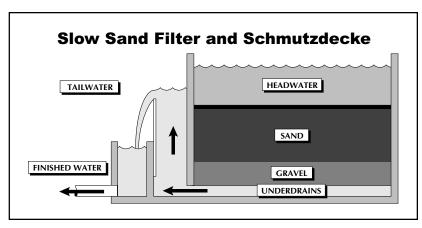
cleaning is used. Slow sand depends on microbes, and their worst enemy is the lack of moisture. The inspector should ask if the filter is ever left unsubmerged and, if so, for how long.
