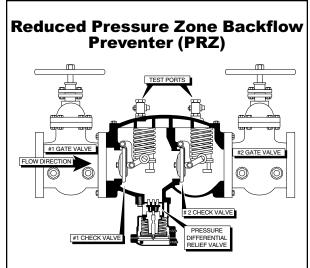
Malfunctioning of one or both of the check valves or the relief valve is indicated by a continuous discharge of water from the relief port; small amounts of water may be periodically discharged during normal operation. Under no circumstances should plugging of the relief port be allowed, because the device depends on an open port for safe operation.
